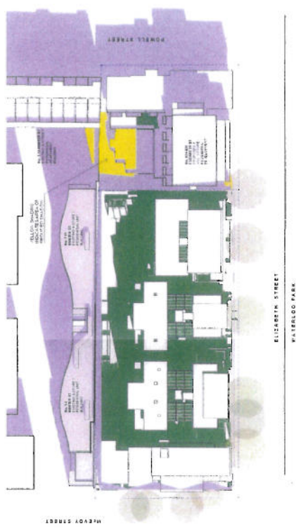
6 21 JUNE 12 PM PROPOSED BUILDING - NTS SHADOW IMPACT ANALYSIS PLAN
